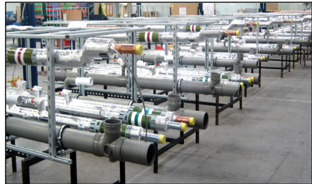
Figure 21 A modularization shop where the components are built in a control environment. Image courtesy of www.mepsolutions.com
