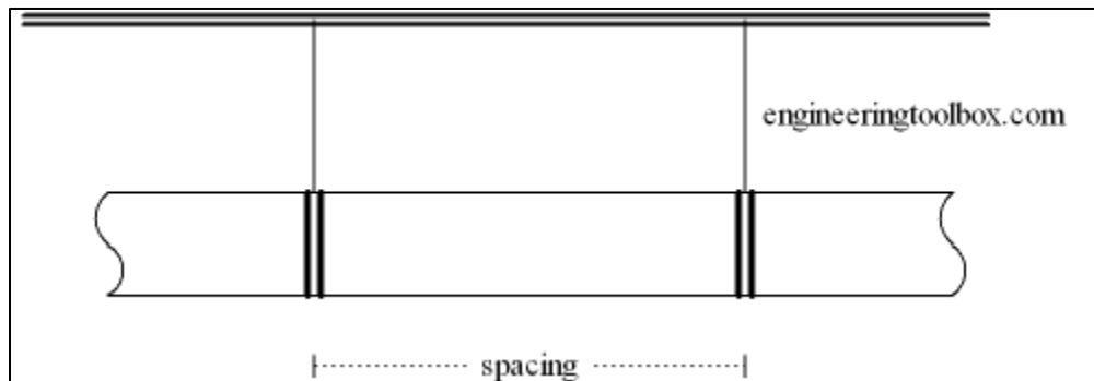
Figure 57 the steel hangers for the MEP system, Image courtesy of www.engineeringtoolbox.com
